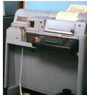
Model 28ASR from Teletype, the Cadillac of RTTY machines in the 1960s.
